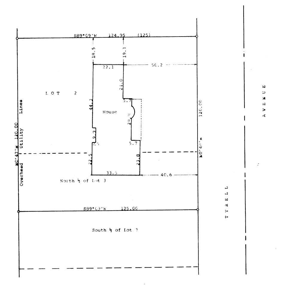
Scale -1" = 20'o = 1" Iron Pipe Found (0.00) = recorded distance Bearings referenced to the recorded bearing of NO°48'W along the west line of Tyrell Avenue. Survey ordered by: Dennis Positano 608 Tyrell Avenue Delavan, WI 53115
